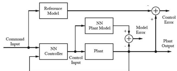
Fig. 1: Model Reference Adaptive Control Architecture
