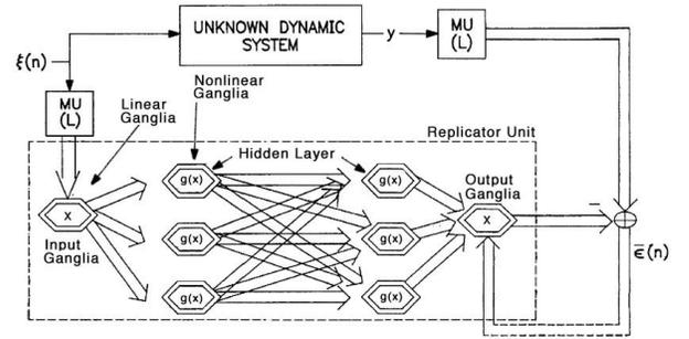
Fig. 8: General Unknown System with Replicator Unit
